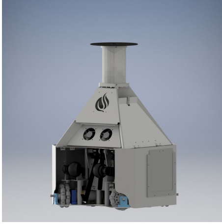
Fig. 1. Third Generation Dagozilla MSL Robot
